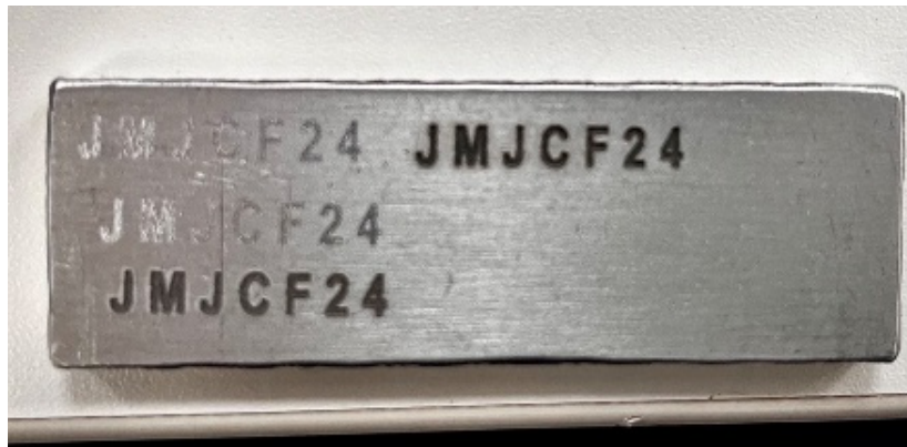
Figure 7 | 304 stainless steel plate with laser engraved markings
