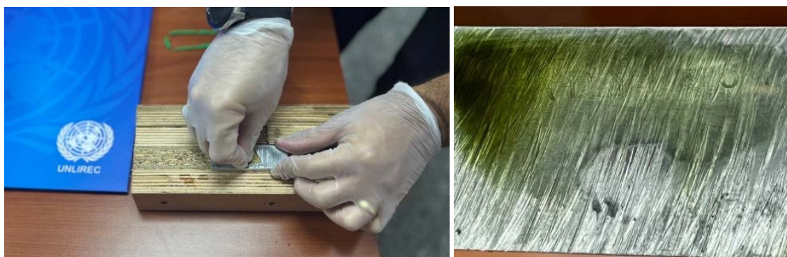
Figure 10 | Chemical etching restoration process
